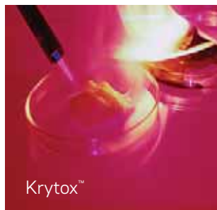
Hydrocarbon-based lubricants burn; Krytox™ does not.
