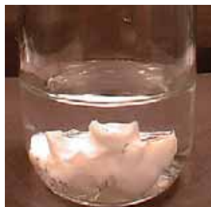
Krytox™ grease in hydrocarbon solvent is not dissolved.
